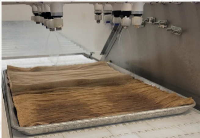
FIGURE 1. The top of crepe cellulose and tray method allows easy application of a constant volume of 700ml of water to each test.
