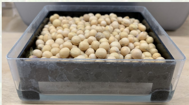
FIGURE 1. Soybean seed placed on AA screen prior to 72 hours of aging, note 40 ml of water below but not touching seed.
