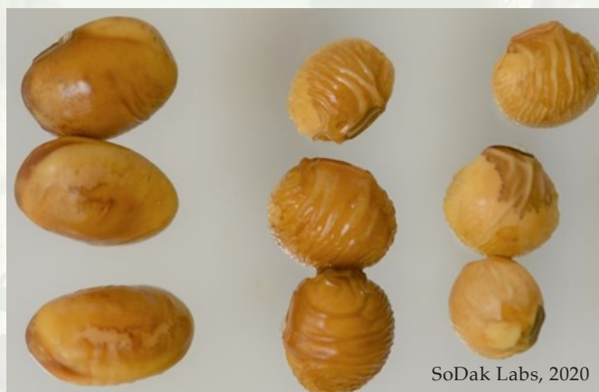
FIGURE 2. Soybean seeds were immersed into hot coffee for three minutes. The swollen oblong seeds on left are damaged. The wrinkle seeds (middle) and firm seeds (right) are considered undamaged.
