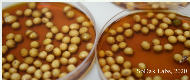
FIGURE 1. Soybean seeds soaking in 60°C (140 °F) coffee to detect physical or mechanical damage to the seed coat.
