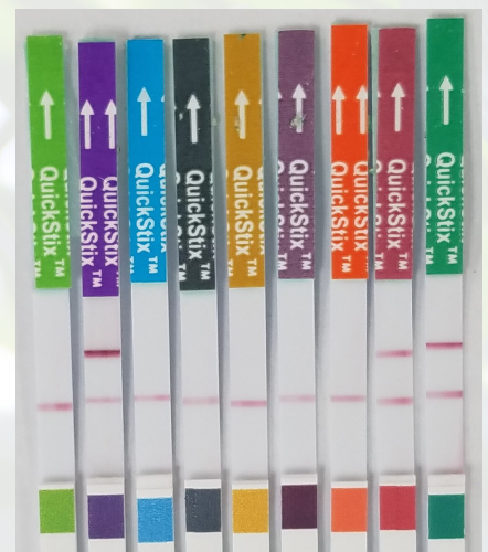
FIGURE 3. ELISA Lateral Flow strip comb showing positive reactions (top marks) and negative reactions for specific traits, as well as control reactions (bottom marks).
