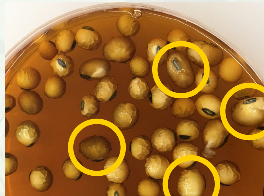
FIGURE 2. Hot coffee soak test, oblong seeds showing seed coat damage
